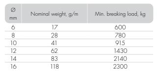
Double braided rope is excellent for mooring, life rings, water rescue or any other use requiring strong rope of light weight and high visibility, specially at night time. Floating.
